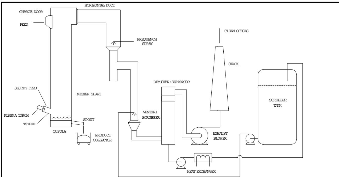
**Figure 2: Plasma Cupola Pilot Plant Schematic**
