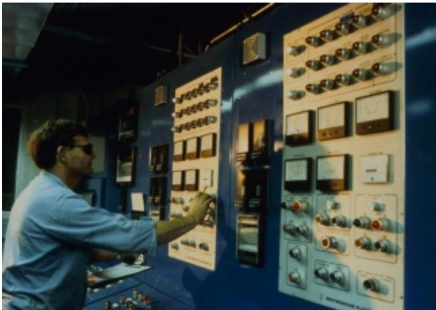
**Figure 4 : Plasma Systems Controls at General Motors Cupola**
