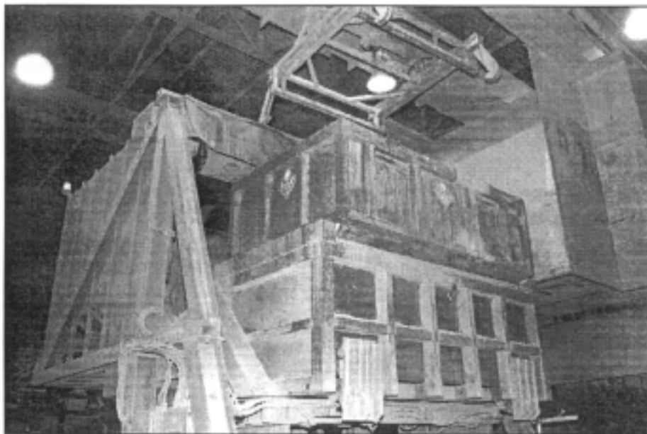
Figure 6 - Container tipper and dust hood.
